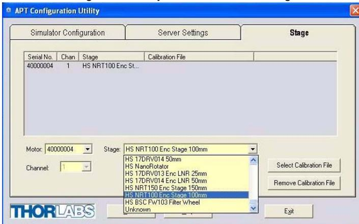
Fig. 3.4 APT Configuration Utility - Stage Tab
