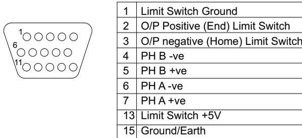
Fig. 4.1 Motor pin out details
