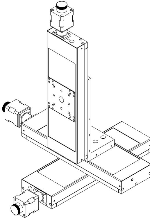
**Fig. 2.1 Typical XYZ Configuration**
