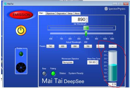
5) Now you are good to use after opening the shutter. For opening the shutter, press and hold the shutter button for 3 seconds
